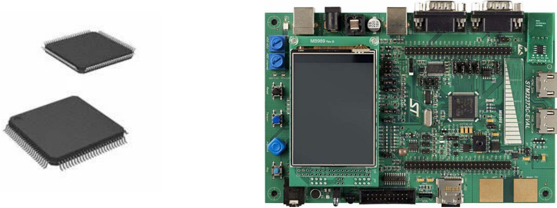
Figure 2. A top and bottom view of the STM32F373VCT6 microcontroller (left) and a top view of the STM32F373VCT6 evaluation board (right) [13], [14].
