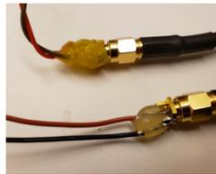
The wire connected to the center pin is then connected to Pin B0 on the evaluation board while the wire connected to the ground pin is connected to Pin B1.
